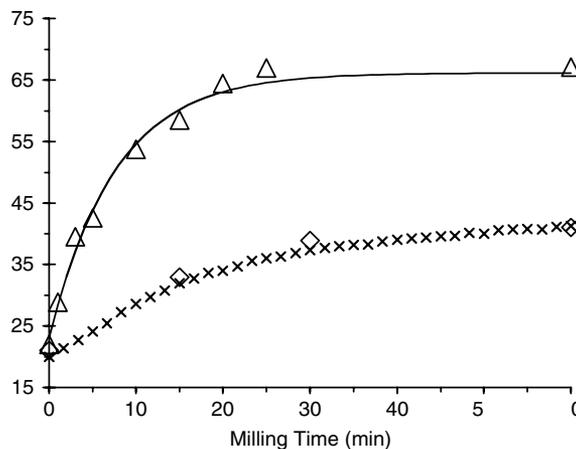
**Fig. 1** Ball temperature as a function of milling time when using a SPEX mill and flat-ended vial with five 12.7-mm balls and no powder (Δ). The continuous line represents a fitted exponential. The temperature of the vial as measured by a thermocouple (×) and independent calorimetric determination (◇) is also shown for comparison
