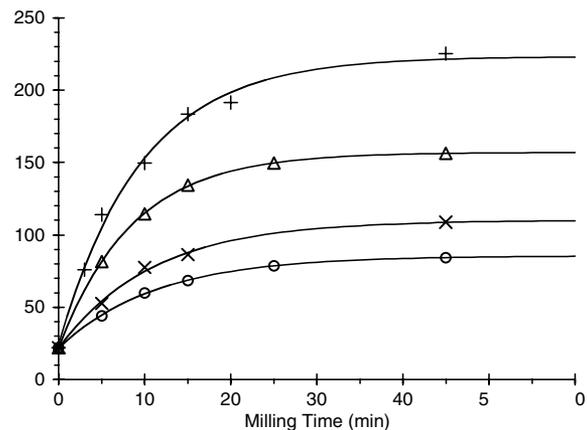
**Fig. 3** Ball temperature—milling time curves obtained using a Fritch P-5 planetary mill. The + and  $\times$  symbols represent data with a 10-cm diameter milling bowl and 100 balls and 280 rpm (+) and 200 rpm ( $\times$ ) speeds and the  $\Delta$  and  $\circ$  symbols correspond to a 7.5-cm bowl, 50 balls and 280 rpm ( $\Delta$ ) and 200 rpm ( $\circ$ ) speeds
