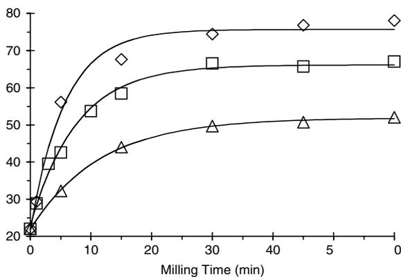
**Fig. 2** Comparison of the ball temperature—milling time curves for a SPEX 8000 mill using five 12.7-mm balls and flat-ended vial with no powder ( $\square$ ), a round-ended vial with no powder ( $\diamond$ ) and a flat-ended vial that also contains 4 g of SiO<sub>2</sub> powder ( $\Delta$ )
