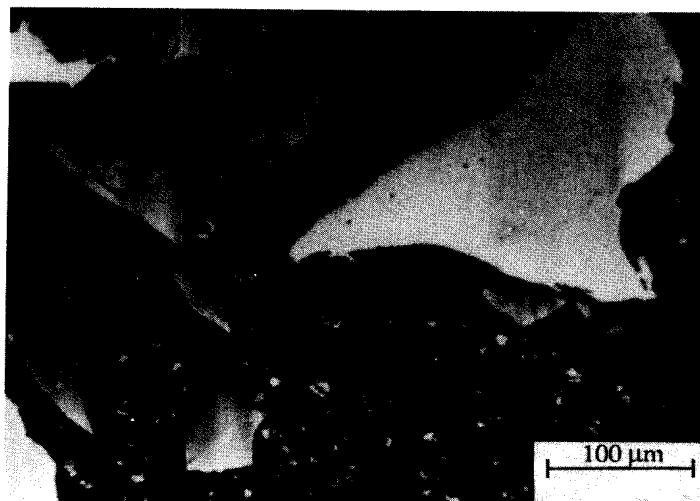
Figure 1 Raw materials for production of a nickel based superalloy: spherical carbonyl nickel (4-7 \mu m), light chromium (50 to 150 \mu m) and nickel-aluminum-titanium master alloy (20 to 100 \mu m). Also present is submicrometer Y_2O_3 not visible at this magnification.
