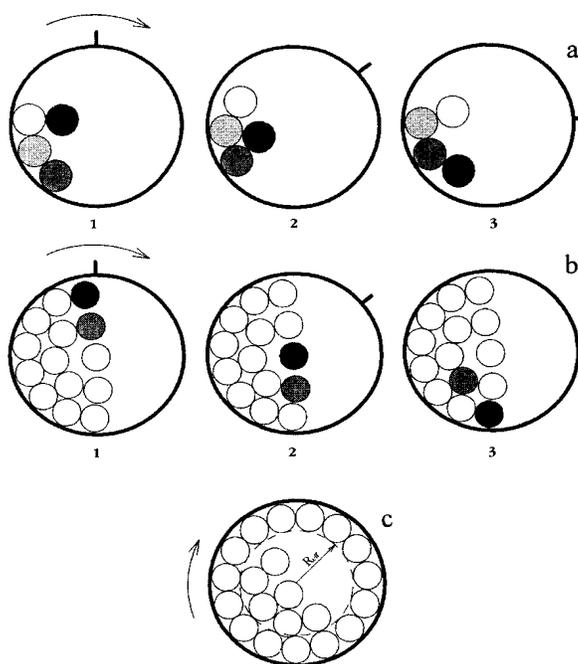
Fig. 1. Schematic representation of ball motion at (a) small (10 - 20 %), (b) medium (40 - 50 %) and (c) high (more than 55 %) values of filled fraction  $\xi$ .
