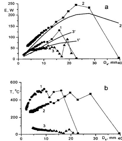
Fig. 3. a - Dependence of E on  $D_b$  at  $\xi$  (%): (1) 15, (2) 45, and (3) 75. (1', 2', 3') - value of E, calculated by equation [16].
