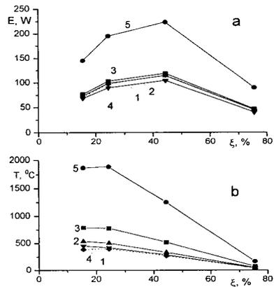
Fig. 4. Dependence of (a) E and (b) T on  $\xi$  for various ball's materials ( $D_b = 8.8$  mm): (1) - Fe; (2) - ShKh-15; (3) - 12Kh18N10T; (4) - Cr; (5) - WC.
