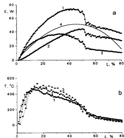
Fig. 2. a - A plot of  $E$  vs.  $\xi$  varied by raising of ball's number from 1 to 121 ( $D_b = 4,8$  mm): (1) - total value of  $E$ ; (2) -  $E_n$ ; (3) -  $E_\tau$ ; (4) -  $E$  calculated by formula [16].
