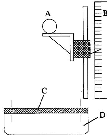
Fig. 3. Experimental set-up for correlation of the indent size with impact speeds by calibrated (B) falls of a ball (A) on to a copper plate (C) supported on a rigid body (D).
