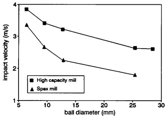
Fig. 5. Impact velocities vs. ball diameter for the high capacity mill and Spex® mill.
