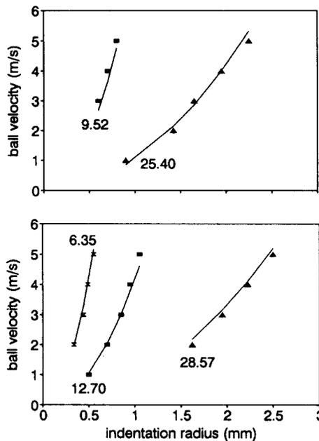
Fig. 4. Correlation of ball (steel AISI 5210) impact velocities with indentation radius (on copper plate) as determined experimentally (points) and with eqn. (1) (continuous lines). Numbers inside the figures are ball diameters (in millimetres).
