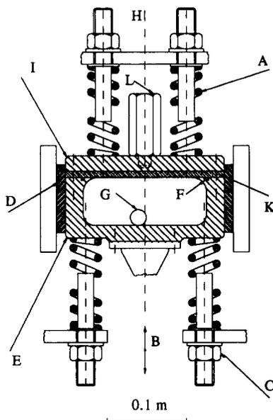
Fig. 2. Section view of the high-energy high-capacity mill: A spring, B driving force (sinusoidal-like), C nut for spring preloading, D Teflon sliding block, E vial, F O-ring, G ball, K copper target plate, I closure plate, L fluids in-out (vacuum, inert or reactive gas), H oscillation axis.
