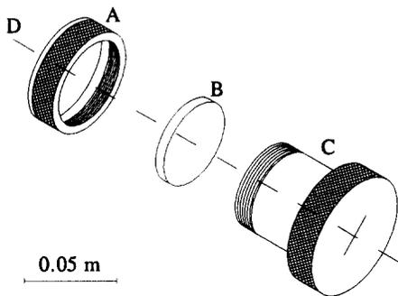
Fig. 1. Exploded view of the vial used in the Spex® mill: A screwed cap, B copper target plate, C vial body with screwed-in cap, D main oscillation axis.
