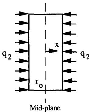
FIG.3 - Approximation of the powder compact as a semi-infinite medium with heat flux conditions at the two impacting surfaces
