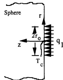
FIG.2 - Approximation of the balls as a semi-infinite medium with constant heat flux condition at a localized area.
