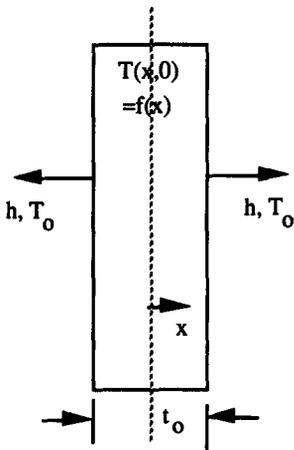
FIG.5 - Dissipation of heat from the powder compact surface during the interval between two impact events.
