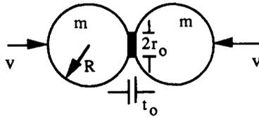
FIG.1 - Geometric parameters involving an impact between powder compact and two balls.
