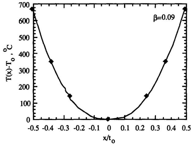
FIG.6 - A typical temperature profile  $T(x)$  across a powder compact thickness impacted with a velocity of  $V=6\text{m/s}$ .
