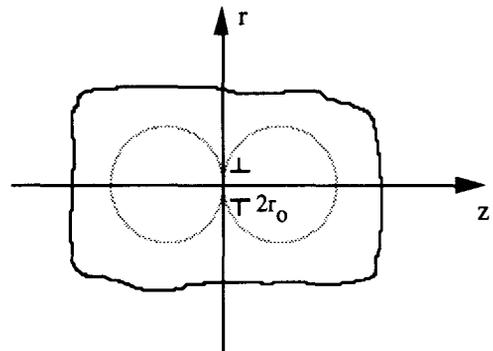
FIG.4 - Approximation of the impact event as an infinite medium with an instantaneous cylindrical surface source at the origin
