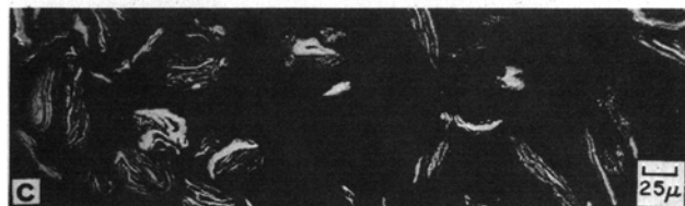
Fig. 5—Structure of powder processed 40 min. (a) Layers welded to ball surface, (b) -80, +100 mesh screen fraction, (c) -325 mesh screen fraction.
