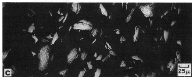
Fig. 6—Structure of powder processed 70 min. (a) Layers welded to ball surface, (b) -80, +100 mesh screen fraction, (c) -325 mesh screen fraction.
